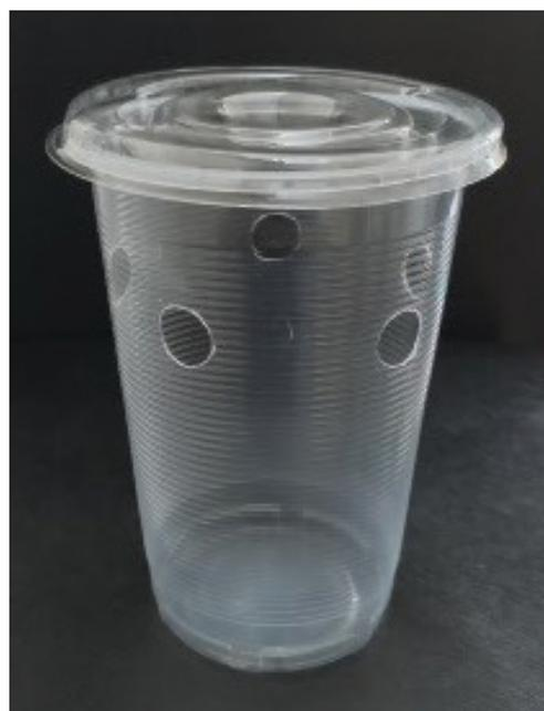
**Figure 2.** Deli cup trap constructed from transparent 370 ml disposable cup (Everpack, Accra, Ghana) by drilling five holes (diameter ~12 mm) equidistant to each other and ~3 cm from the top of the cup
